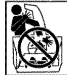
DANGER Stop The Engine Before Unclogging Discharge Chute!
