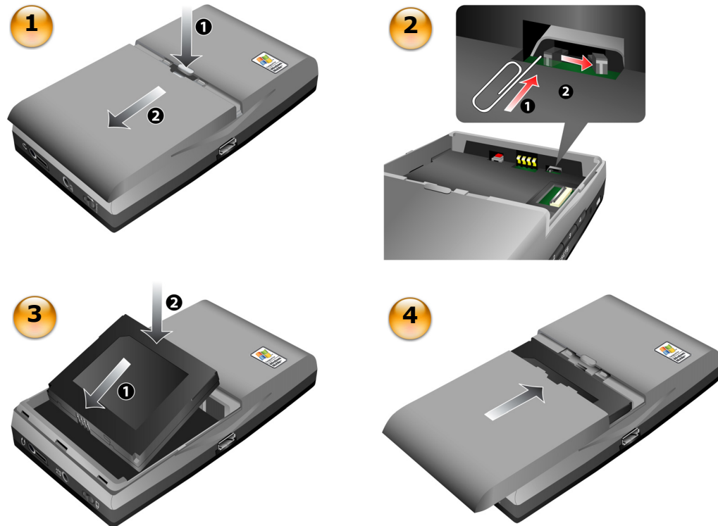
Figure 3-1: Inserting the battery in your Zen Portable Media Center
