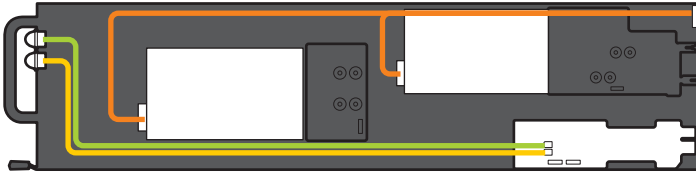
Figure 3-10. Cable Routing for PSU1/3 Module Assembly
