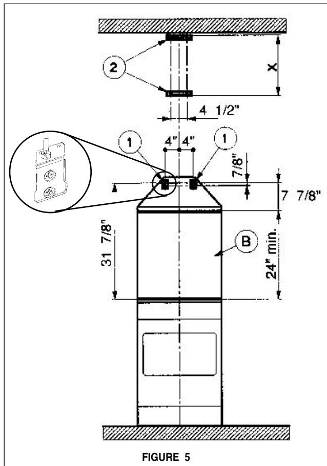
4. The chimney mounts by two brackets (**Item 2 in FIGURE 5**). Note the position of the brackets. The top bracket should be installed about 1/8" away from the ceiling. The bottom bracket must be installed at the bottom point of the upper chimney sleeve.
