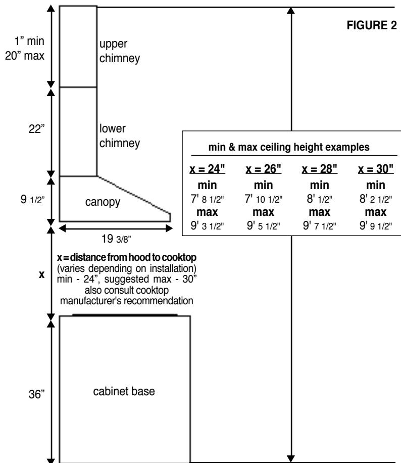
For shorter ceilings, have the chimney cover(s) cut at a sheet metal shop. For higher ceiling installations, the **High Ceiling Chimney Kit** includes a new 40" upper chimney which would replace the 20" upper chimney that came with the hood. (see **OPTIONAL ACCESSORIES page 4**)
