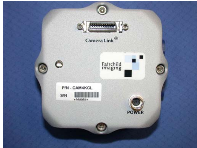
Figure 2.2-1 MDR-26 CameraLink™ Connector 3M p/n 334 – 34 series
