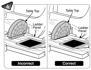
Check to be sure the table top is properly attached to the ladder panel. There should be no gap between the table top and the ladder panel.
