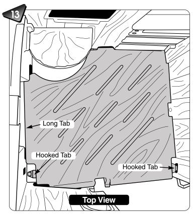
Insert and snap the hooked tabs and long tab on the platform into the panel assembl, as shown.
