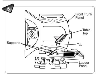
Position the assembly so that the ladder panel is laying on a flat surface.
