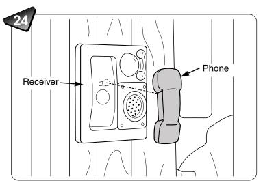
• Fit the phone into the receiver on the wall panel.
