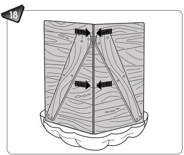
• Fit the hooked tab and the long tab on the left roof into the slot and groove in the right roof.
