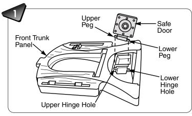
Position the front trunk panel on a flat surface with the inside facing up.
