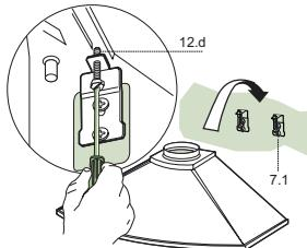
**Note:** The Hood body should be secured to wall studs. If necessary, install a wood support behind the dry wall, flush mounted between 2 studs. This will provide the necessary structure and support for mounting.
