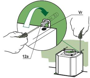
**Note:** The Hood body should be secured to wall studs. If necessary, install a wood support behind the dry wall, flush mounted between 2 studs. This will provide the necessary structure and support for mounting.
