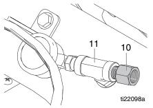
6. Apply pipe sealant to hose (99) and screw into filter fitting (10). Screw in until gas tight.
