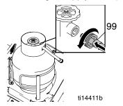
8. Open manual gas shutoff valve on propane.
