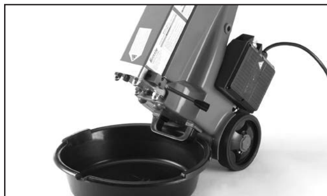
Figure 11. Draining hydraulic fluid.
