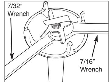
2. While holding the shaft in place, use a  $7/16$ " wrench to turn the blades **clockwise** to loosen the blades.
