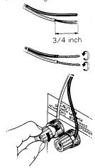
**CAUTION**: Two speaker systems can be connected to this unit. The minimum speaker impedance should be 4 Ohm when only one speaker system is connected. When two speaker systems are connected, care should be taken that net impedance does not become less than 4 Ohm.
