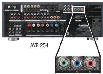
Figure 33 – Component Video Monitor Outputs
