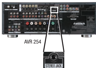
Figure 30 – Connecting a Portable Audio Player
