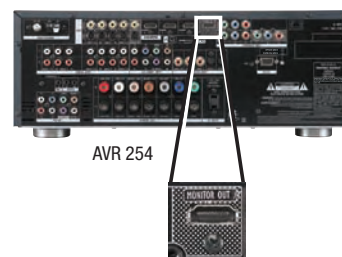
Figure 32 – HDMI Monitor Output
