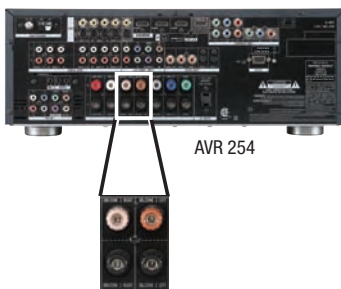
Figure 39 – Surround Back/Zone 2 Speaker Outputs
