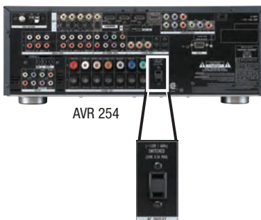
Figure 35 – Switched AC Accessory Outlet
