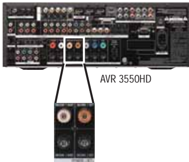
Figure 43 – Surround Back/Zone 2 Speaker Outputs
