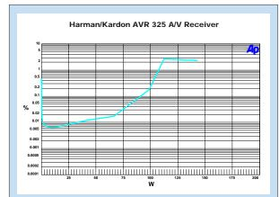
HT Labs Measures: Harman/Kardon AVR 325 A/V Receiver This graph shows that the AVR 325's left channel, from CD input to speaker output with two channels driving 8-ohm loads, reaches 0.1% distortion at 90.4 watts and 1% distortion at 107.2 watts. Into 4 ohms, the amplifier reaches 0.1% distortion at 135.2 watts and 1% distortion at 156.9 watts. With five channels driving 8-ohm loads, the amplifier reaches 0.1% distortion at 73.8 watts and 1% distortion at 84.5 watts.
