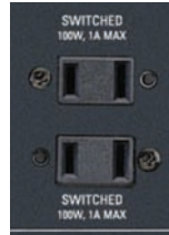
Figure 21 – Switched AC Accessory Outlets
