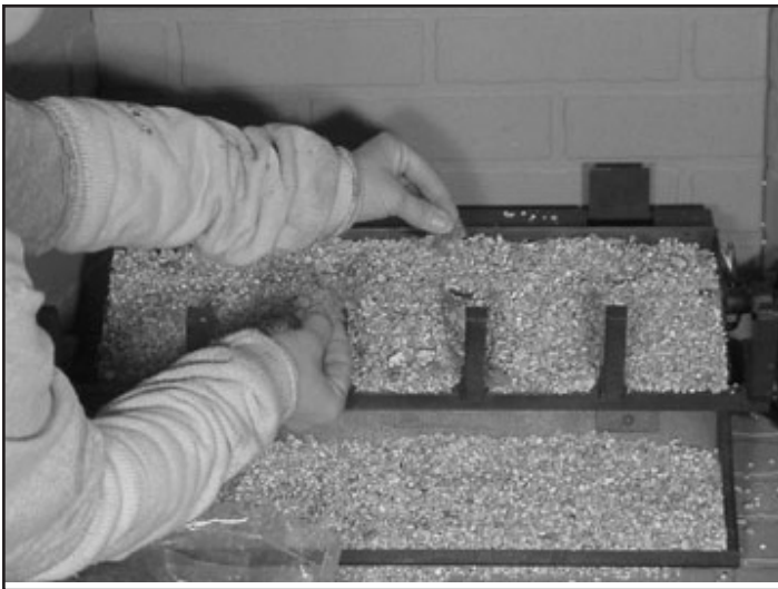
Figure 5 Placing Rock Wool
