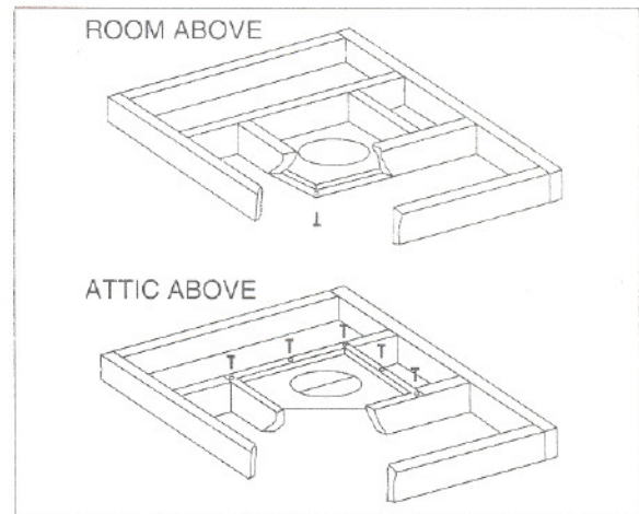
Figure 13 Installing the firestop spacer
