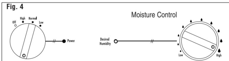
**NOTE:** If the humidifier fan will not start or restart when you select a fan speed, the Moisture Control may be set too low. Turn the dial clockwise ↗ to the largest raindrop (💧) before High. The Desired Humidity Light will be Off when the unit is producing moisture (Fig. 4).
