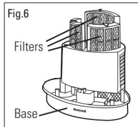
**NOTE: REMOVE FILTERS BEFORE CLEANING.
