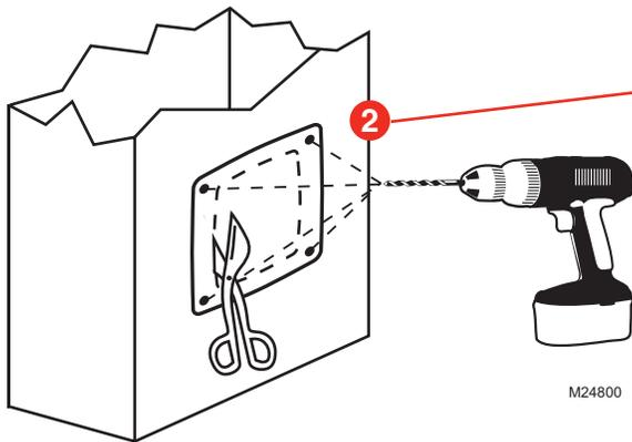
2 Apply sticker template to duct and drill holes for mounting screws. Cut along the dotted line of the template with metal shears or tin snips.
