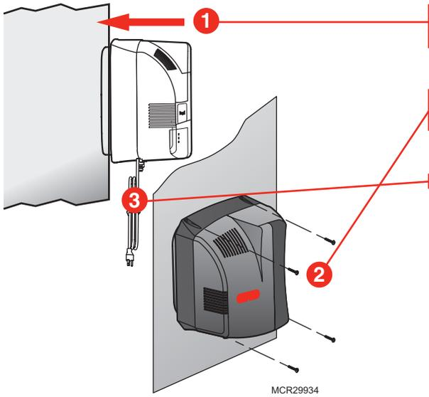
Slide the Fan model evenly into the duct hole. Verify the humidifier is level.
