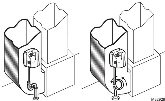
If a return duct installation is required, a trap must be installed in the drain line. A hard trap is recommended, but a coil in the line, secured with tape or zip tie, is also acceptable.
