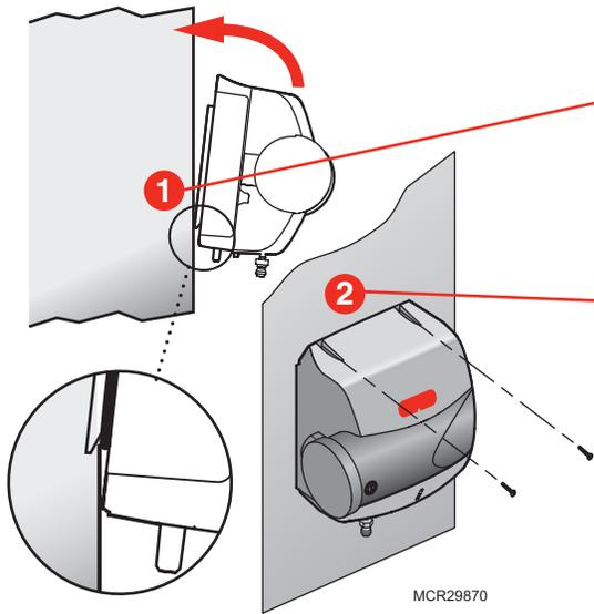
Secure the support hooks on Bypass models to the bottom lip of the hole.
