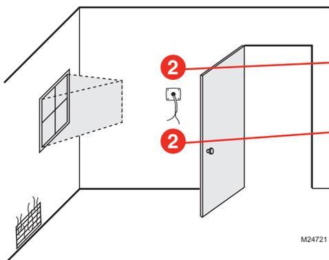
Cut 1-in. diameter wire hole in wall.
