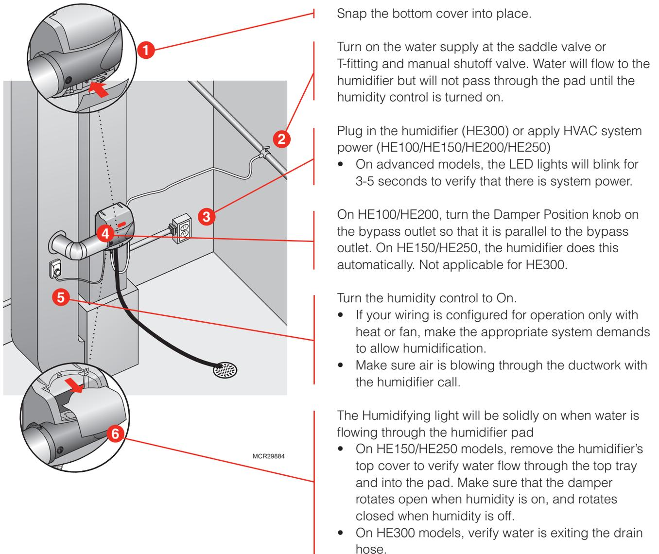
Check all water line and drain connections to ensure there are no leaks before leaving the job site.
