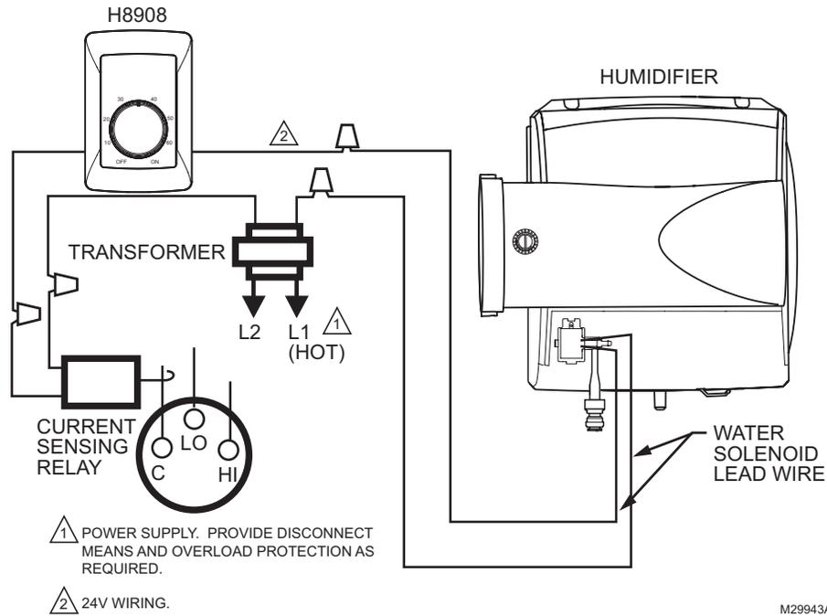
Wiring H8908 in line with air proving device.
