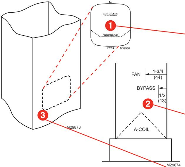
Position the template on the duct.
