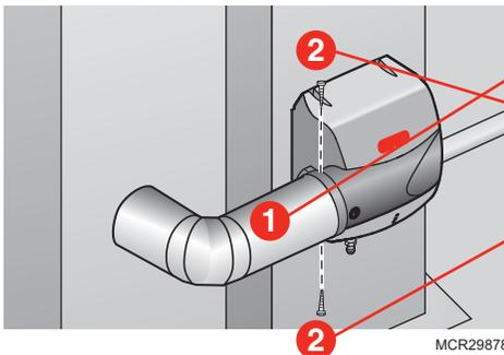
Use rigid or aluminized flexible 6-in. duct to connect the starter collar to the humidifier bypass port.
