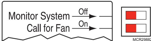
**DIP 1 (Top):** This switch looks for inputs from the HVAC system before allowing humidity. Set to the left, the humidifier will look for input(s). Set to the right, it will not.
