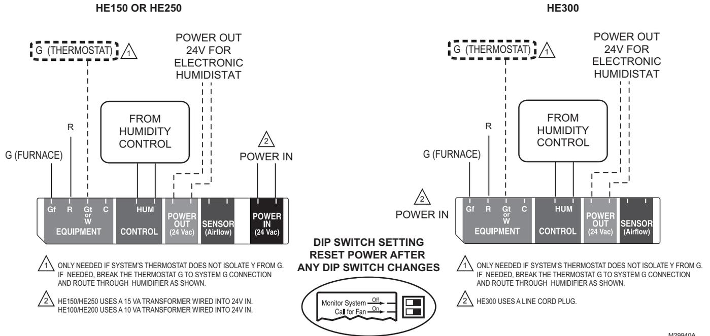
Wiring to force fan on and prove airflow in the duct.
