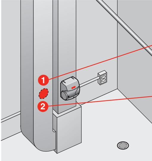
On the duct opposite the humidifier Bypass install, cut a 6-in. diameter duct hole.
