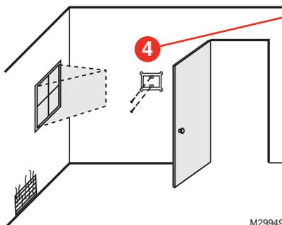
Secure the base bracket to the remote location with two 1-in. (25 mm) screws (provided).
