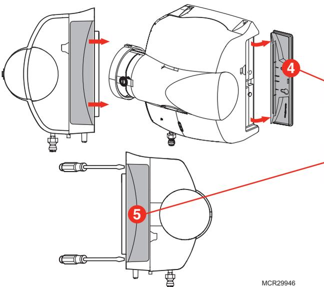
Ensure that the pad is accessible. The handle of the pad holder and side panel of the humidifier can be switched so the pad holder can be removed (opposite side of the bypass duct opening).
