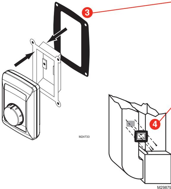
3 Remove the base bracket from the humidistat. Slide the black gasket onto the base bracket.
