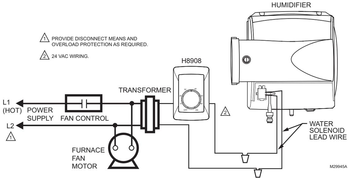
Wiring H8908 with 2-speed fan motor.
