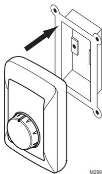
Remove the base bracket from the humidistat.
