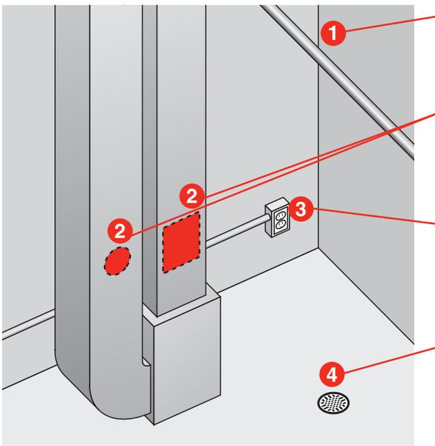
Choose a location that has access to a water supply pipe. Cold or hot water can be used.
