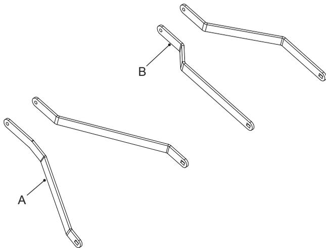
2. Install the bagger mount tube to the rear guard with  $\frac{5}{16}$ -18 x  $3\frac{1}{4}$  bolts and flange nuts from kit.
