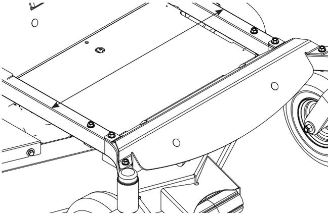
For frames measuring 26" use support straps A, for frames measuring 23" use support straps B.
