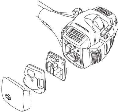
An oiled foam plastic filter (available as an accessory) must be used if the machine is operated in extremely dusty conditions. See instructions under the heading Oiling the air filter.
