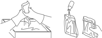
An air filter that has been in use for a long time cannot be cleaned completely. The filter must therefore be replaced with a new one at regular intervals. **A damaged air filter must always be replaced.**
