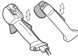
Check that the throttle control and throttle lockout move freely and that the return springs work properly.
