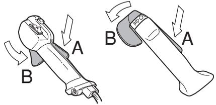
Make sure the throttle control is locked at the idle setting when the throttle lockout is released.
