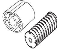
Regularly check the vibration damping units for cracks or deformation. Check that the vibration damping element is undamaged and securely attached.
