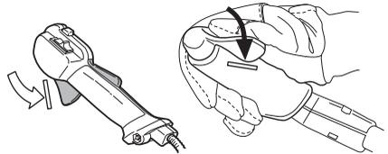
Press the throttle lockout and make sure it returns to its original position when you release it.
