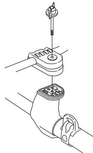
Fit the right handle to the handlebar using the screw, washer, sleeve and nut as shown. Tighten.
