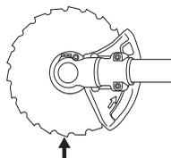
When loosening and tightening the saw blade nut, there is a risk of injury from the teeth of the saw blade. You should therefore always ensure that your hand is shielded by the blade guard when doing this. Always use a socket
