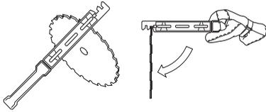
Check the cutting attachment for damage or cracks. A damaged cutting attachment should always be replaced.
