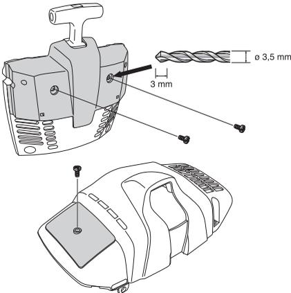
These reduce the cooling air and prevent large amounts of snow from being sucked into the engine.
