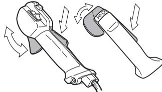
See instructions under the heading Start. Start the machine and apply full throttle. Release the throttle and check that the cutting attachment stops and remains at a standstill. If the cutting attachment rotates with the throttle in the idle position then the carburettor idle setting must
